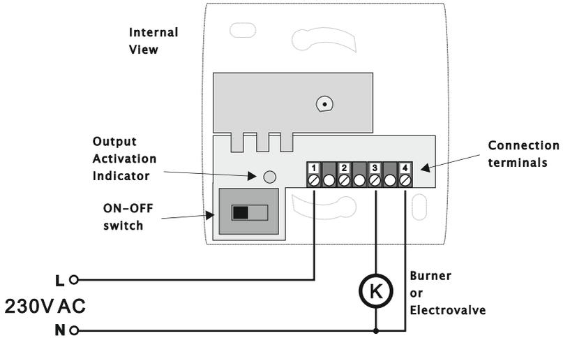
Figure 1. Connection diagram
